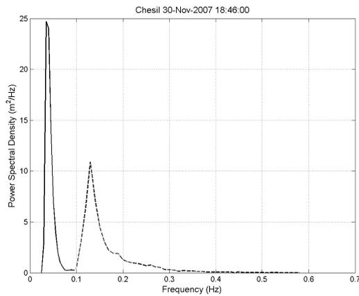
**Figure 1.** 1-D spectrum from a Directional Waverider in ~12m water depth off Chesil Beach. Total  $H_s = 3.84\text{m}$ , 44% of the energy is in a well-defined, narrow, low frequency component.
