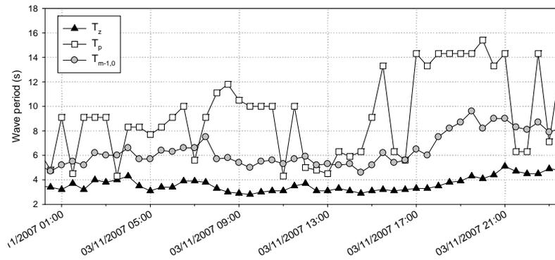
**Figure 11. Time series of wave period parameters, including Eq. (1), at Hayling Island.**
